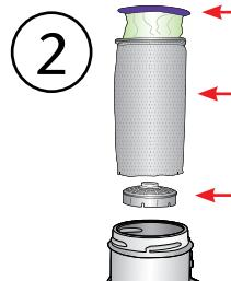
Check to make sure the filters are in place and have not shifted during shipping.
