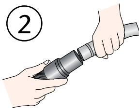
Twist the wand onto the end of the hose.
