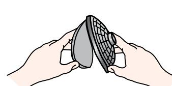
Pull the top piece of the Dome Filter off and remove the foam media. Shake it out, rinse it, and let it air dry thoroughly. HEPA MODELS: For best results replace pleated Dome Filter every 6 months (or more often if necessary).
