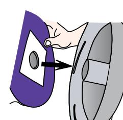
For vacuums with closed top bags, slide the gasket of the filter over the inlet on the inside of the top cap, then replace the cap.
