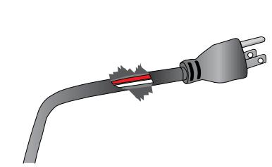
DO NOT vacuum with a frayed, worn or damaged cord. Do not modify the vacuum plug. Use the extension cord provided.
