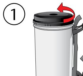
Unscrew the cap on the top of the vacuum unit.
