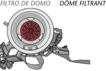
Once a week, or as necessary, clean or replace the Dome Filter. First, remove the Intercept Micro Filter and Cloth Filter. Reach into the vacuum body and twist Dome Filter from motor.
